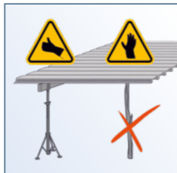
9 - Use a suitable prop equipment
