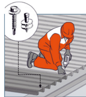
14 - Fix profiles sheets on supports and stitch them among each other (2 fixings per profile sheet and per end support)
