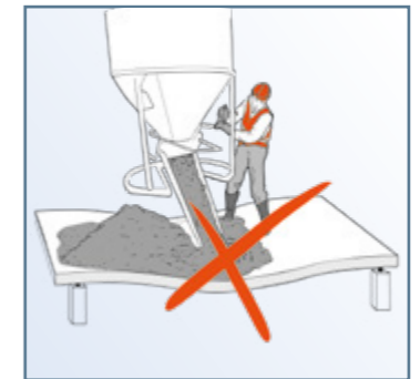
19 - Avoid any concrete accumulation while concreting
