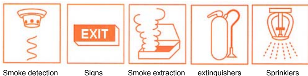
Figure 6.4 Active fire protection methods
